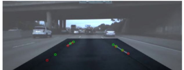
Fig. 4. Visualized feature points detected on the masked image using OpenCV.
