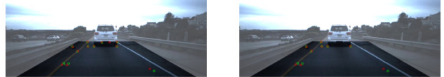
Fig. 7. Frame 1 of the validation dataset. Using the polygon mask results in keypoints placed on a close vehicle. Taking the pixel-wise or of the segmented road and original polygon mask results in more suitable keypoints being selected.
